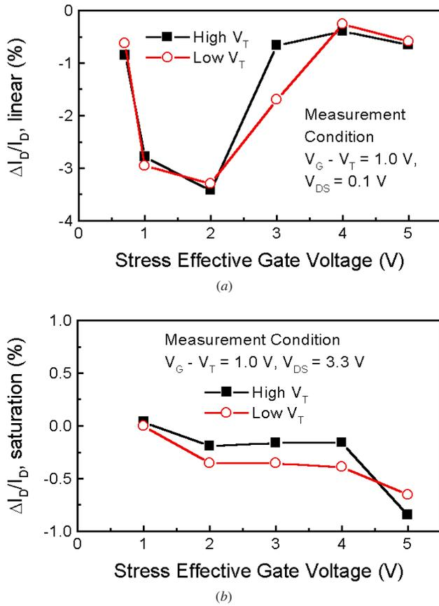
**Figure 1.** Drain current mismatch at the (a) linear and (b) saturation regions of NMOSFETs ( $W_{\text{gate}}/L_{\text{gate}} = 3.0/2.0$ ) as a function of stress effective gate voltage. The threshold voltages for high  $V_T$  and low  $V_T$  devices are 0.7 and 0.4 V, respectively. Stress was achieved for 30 min at  $V_{\text{DS}} = 5.0$  V.
