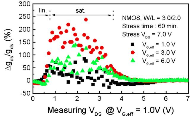
**Figure 2.** The variation of output conductance depending on stress effective gate voltage. The output conductance was measured at  $V_{\text{G,eff}} = 1.0$  V and at the whole drain voltage. The stress time is typically 60 min.
