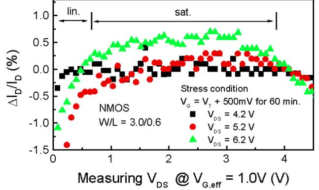
**Figure 4.** The variation of drain current depending on stress drain voltage. The drain current was measured at  $V_{G,\text{eff}} = 1.0$  V and at the whole drain voltage. The stress time is typically 60 min.
